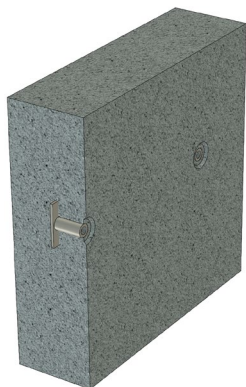
Solid wall with cast-in anchors.
