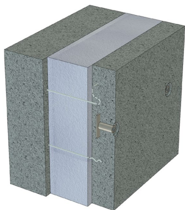
Sandwich wall with cast-in anchors in outer panel.
